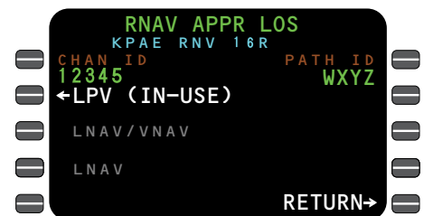
SBAS-FMS Approach Mode provides ILS-like guidance with LPV, LNAV/VNAV and LNAV level of service for RNAV (GPS) approaches.
